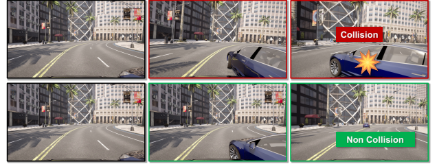
Figure 5: Closed-loop case in CARLA. The top row shows Vanilla DriveLM producing an unsafe maneuver that leads to a collision, while the bottom row shows DriveLM+LATENTGUARD repairing the unsafe latent state and generating a collision-avoiding decision.
