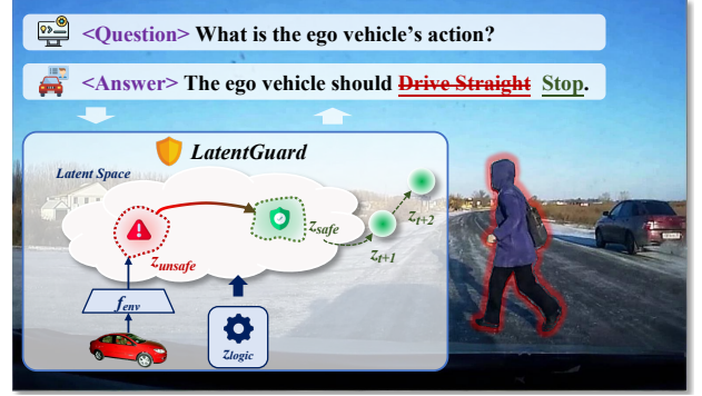
Figure 1: Illustration of LATENTGUARD. LATENTGUARD repairs unsafe AD-VLMs responses by shifting the latent representation from an unsafe state to a safer world-consistent state.
